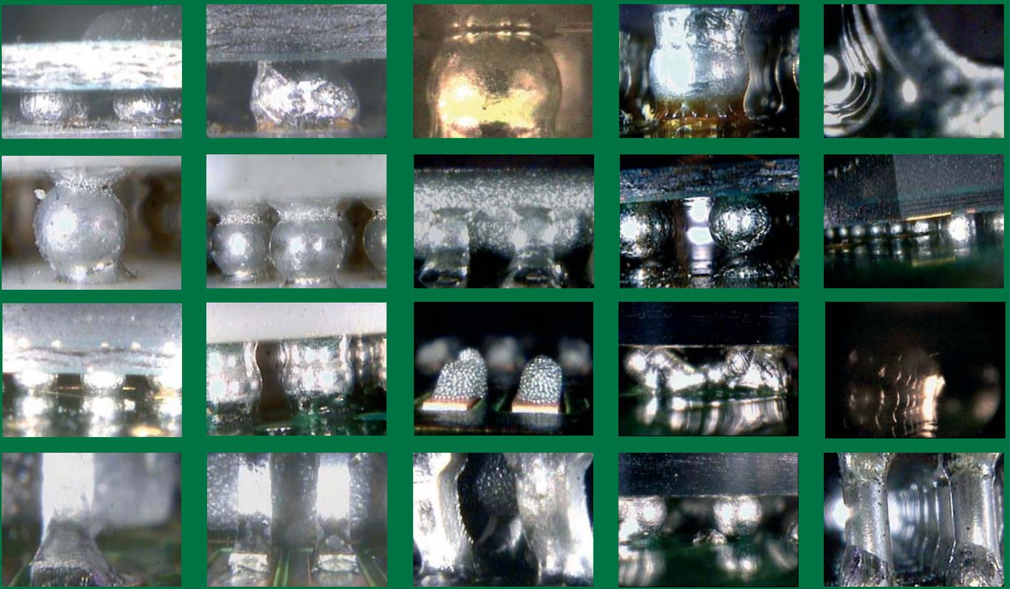
**The endoscopic inspection system BGA.Inspector permits a comfortable control of electronic components, from BGAs to flip-chips.**
