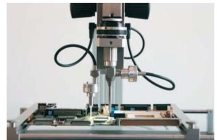
BGA.Inspector with endoscope
